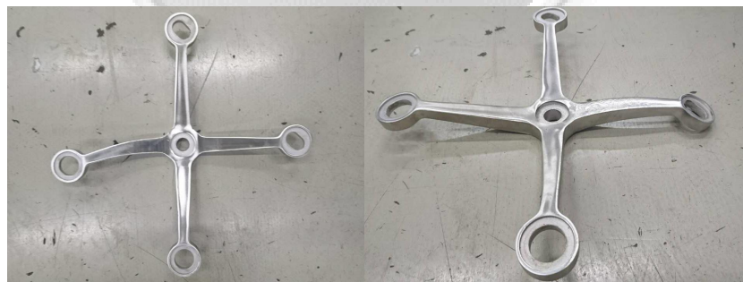
Photo. 6: Mode of failure - Spider fitting
